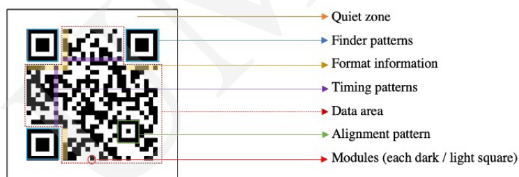
Figure 1. Elements of a QR code symbol
