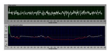
Fig. 4. The charts of the network delays for the VoIP traffic with a heavy load and the Hurst exponent value obtained using the absolute value method.
