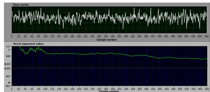
Fig. 6. The charts of the VoIP traffic with a heavy load and the Hurst exponent value obtained using the absolute value method.
