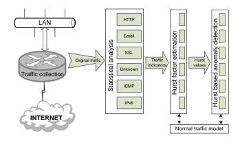
Fig. 1. Network traffic anomaly detection scheme
