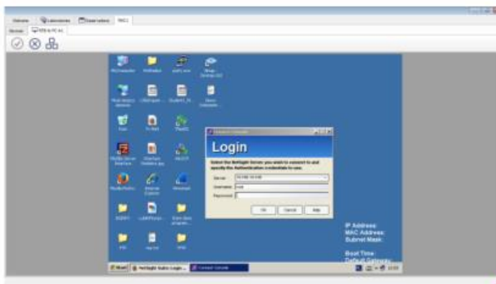
Figure 4 VNC access to a remote virtual PC
