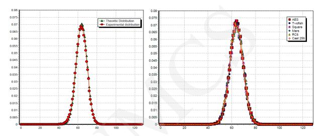
FIGURE 4. Distribution of output's sensitivity to plain-text variations: (a) theoretic distribution versus experimental distribution of the proposed block cipher, (b) experimental distribution of some popular block ciphers.
