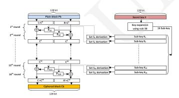
FIGURE 3. Pictorial description of the proposed block cipher.
