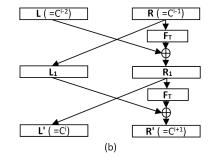
FIGURE 2. Equivalence between RCA's mechanism and Feistel functions :(a) two iterations of RCA; (b) two Feistel rounds.
