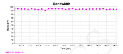
Fig. 2. 100 Mbit/s link test measurements.
