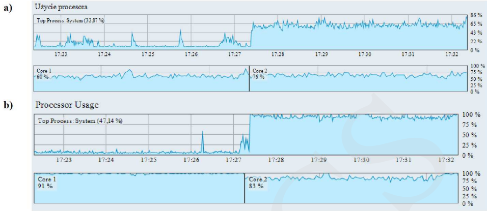
Fig. 9. The CPU usage for the VPN tunnel with PPTP/IPsec in FastEthernet: a) server; b) client.
