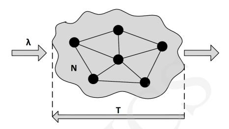
Fig. 2. Graphical representation of Little's law for the system in the steady state.
