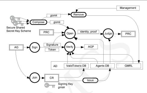
Fig. 2. Revocable Anonymity System's Architecture.
