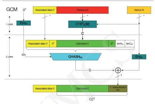
Fig. 6. GCM authenticated encryption scheme.
