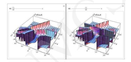
Fig. 2. Dedependence between the mass m1, distances  $\alpha, \beta$  and angular velocity  $\omega$  where  $m1 \in [0.00001, 0.1]$  (the slider represents the values of m1),  $\alpha \in [0.0001, 2], \beta \in [0.0001, 2].$
