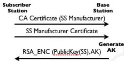
Fig. 4. Station Authentication Process.
