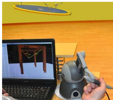
Fig. 9. The control of the cable manipulator system by means of the haptic.
