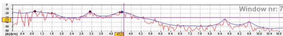
Fig. 1. Spectrum (in decibels) of vowel 'a' Smooth curve is obtained by Linear Prediction and the more frequency-varying one is obtained by the Fourier analysis. The sampling rate is 22kHz.
