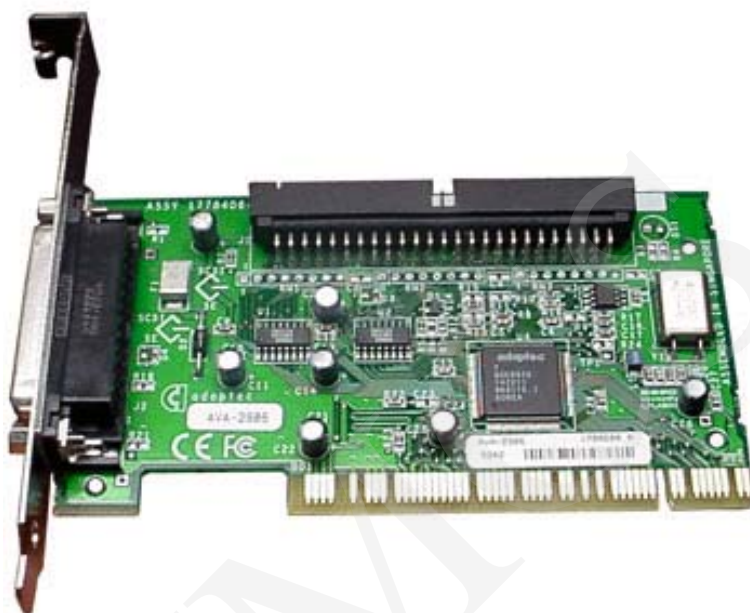
Fig. 2. Adaptec AVA 2906 controller.
