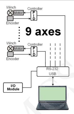
Fig. 5. The architecture of control system
