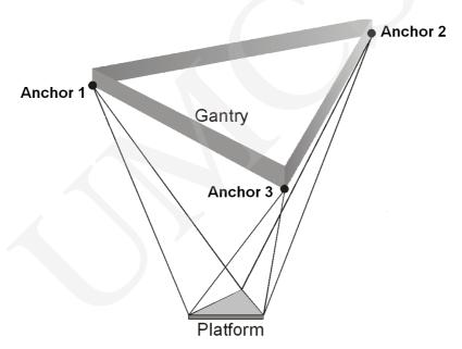
Fig. 2. Six DOF robotic crane - NIST RoboCrane®
