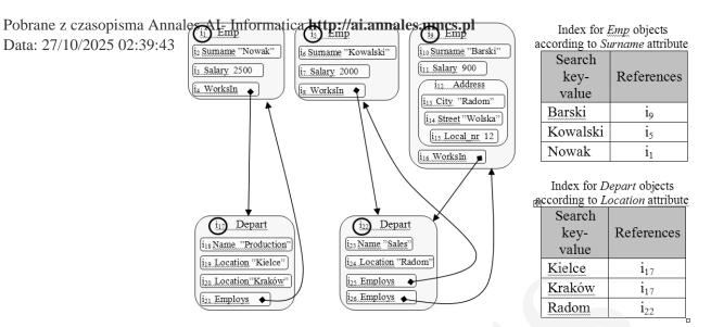
Fig. 2. Example of dense indices for a given object-oriented database store
