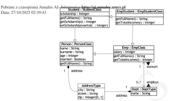
Fig. 3. Example object-oriented schema
