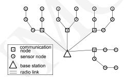
Fig. 2. Sensor network with communication nodes
