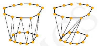
Fig. 5. Contour stitching – tailing. On the left side correct connections; on the right side causing bending of surface
