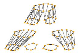
Fig. 6. Contour stitching – branching. On the top the correct connection of contours, while in the bottom line wrong solutions
