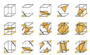
Fig. 2. The marching cubes triangulation classes used in the marching cubes algorithm.
