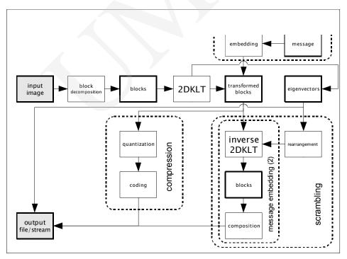
Fig. 2. General diagram of 2DKLT-based image processing algorithms
