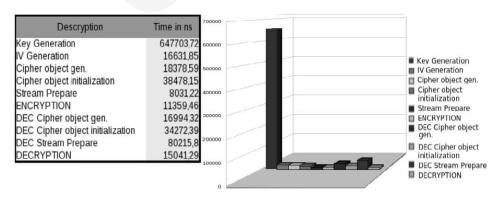
Fig. 6. Time consumption of the Triple DES algorithm
