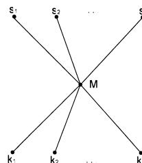
2) *Multichannel bus (tripartite graph)*. Improvement of the single-channel bus in the sense of raising SK reliability is a multichannel bus. The graph lying at the basis of this topology is the tripartite graph (Fig. 2), where  $s_1, s_2, \dots, s_r$  – servers,  $k_1, k_2, \dots, k_n$  – computers,  $M_1, \dots, M_m$  – buses.
