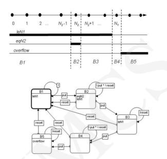
Fig. 2. CSM model of Buffer for  $N_1 > N_2$
