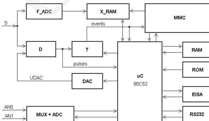
Fig. 2. Block diagram of random events recorder
