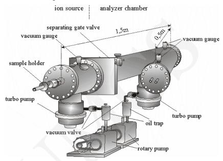
Fig. 2. The vacuum system of the TOF spectrometer
