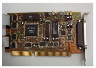
Fig. 3. The analog-digital card ADC615
