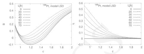
Fig. 1. Deformation parameters corresponding to the fission path of <sup>188</sup>Pt
