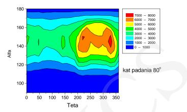
Fig. 2. Contour plots (lines of equal intensity) of the angular distribution of sputtered particles for N->Ti (1500eV) and angle of incident  $\phi$ =80<sup>0</sup>
