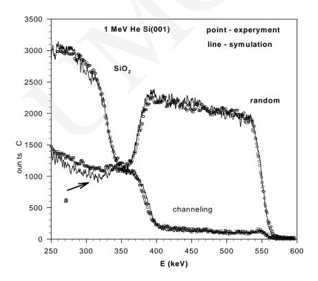
Fig. 3. Experimental [13] and simulation RBS energy spectra for SIMOX structure
