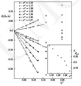
Fig. 5. The energy contribution due to the crossing of heavy walls as a function of  $l_x^{-1}$  for a series of systems characterized by  $e_y = 1.0$ ,  $V_b = 1.0$  and different size of adsorbate atoms (shown in the figure). The inset shows the plot of  $e_{cro}^*$  versus  $s^*$
