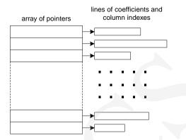
Fig. 1. New storage structure of sparse matrix using the array of pointers and dynamic lines
