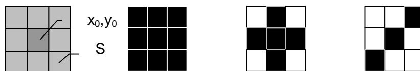
Fig. 1. Structuring element with labeled origin and most commonly used neighborhood shapes
